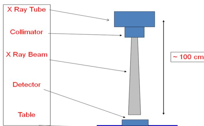
**Figure 2.** The position of detector for measurement
