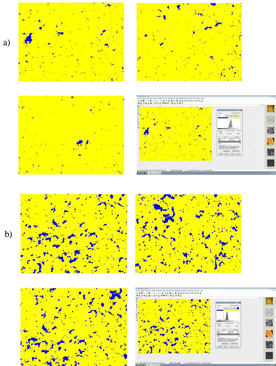
**Figure 2.** Three of the photos (magnification 100X) examined with View-7 image analysis software for the a) Albanian-Dalmatian axe sample and b) celt axe sample. Pores and alloy differ in colors (pores are blue, the alloy is yellow) which can be chosen in the software settings.
