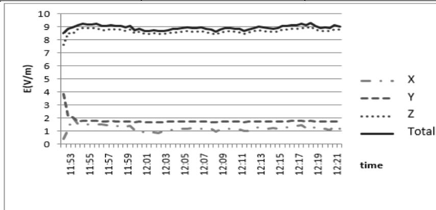
**Figure 6.** The intensity of the electric field, measured in the computer lab between two computers, when all the computers are switched on, as a function of time.
