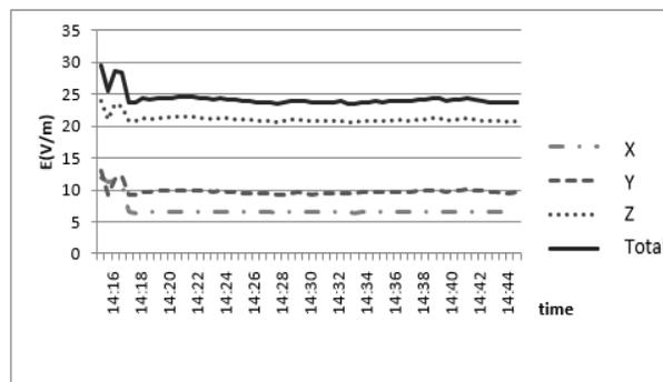
**Figure 3.** Variation with time of electric field intensity E (V/m), in front of the box at 50 cm distance from the box, at the height of standing position (170 cm). Computers are switched off.
