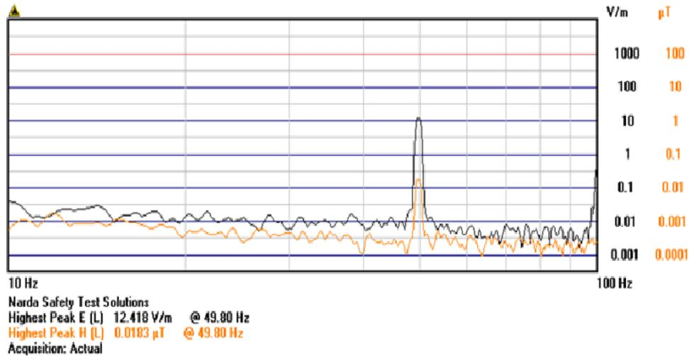
**Figure 4.** Actual acquisition of electrical and magnetic fields, 50 cm outside the box on the left, at the height of sitting position. Computers are switched off.
