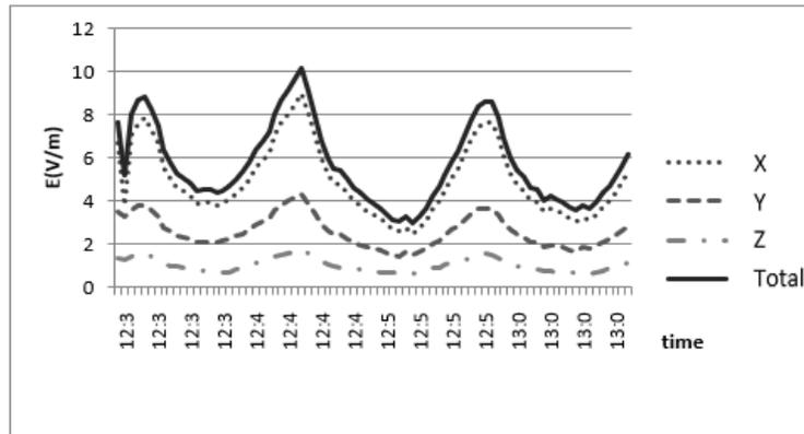
**Figure 5.** Variation with time of electric field intensity  $E$  (V/m), inside the rack mount where is kept the central server of PUT.
