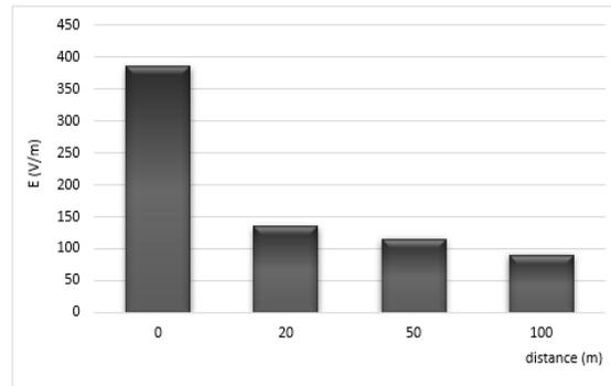
**Figure 2.** Variation of electric field intensity E (V/m), with distance from the box.
