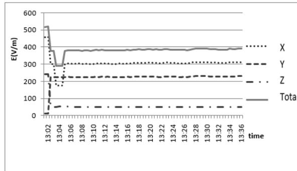
**Figure 1.** Variation with time of electric field intensity E (V/m), inside the box where the switch is kept.
