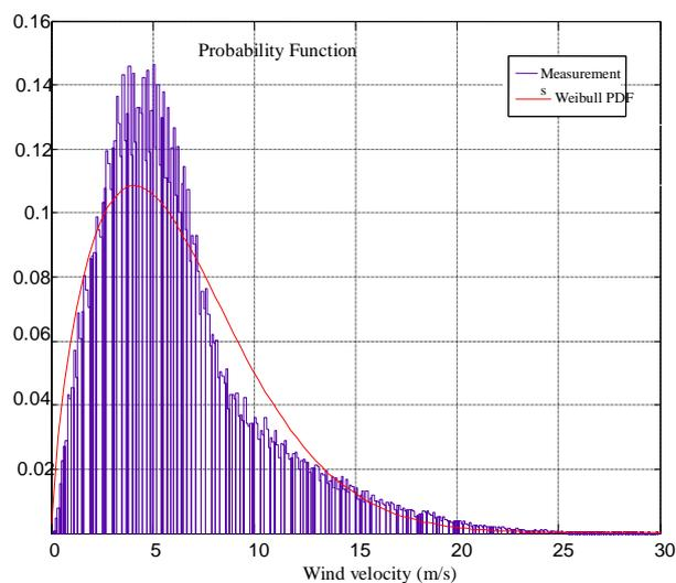
**Figure 2.** Weibull probability function and measurements
